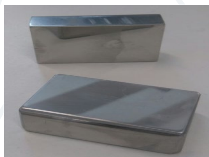
Polished samples taken from the LMD overlay and used in the ASTM G48 corrosion test
