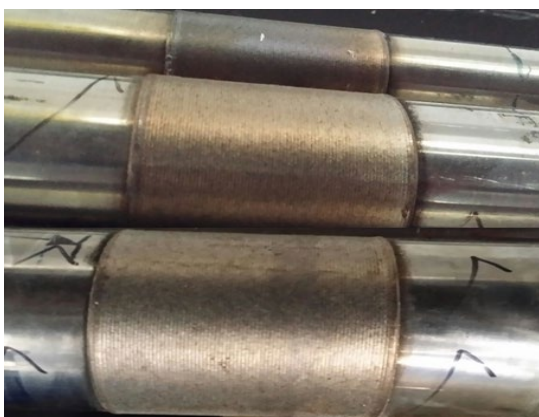
LMD overlay on a critical feature that is damaged in service on a pump shaft
