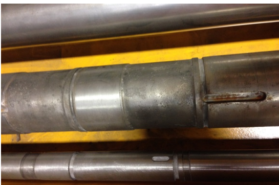
Wear damage on pump shafts
