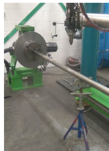
LMD overlay stage on the round bar - representative of a pump shaft
