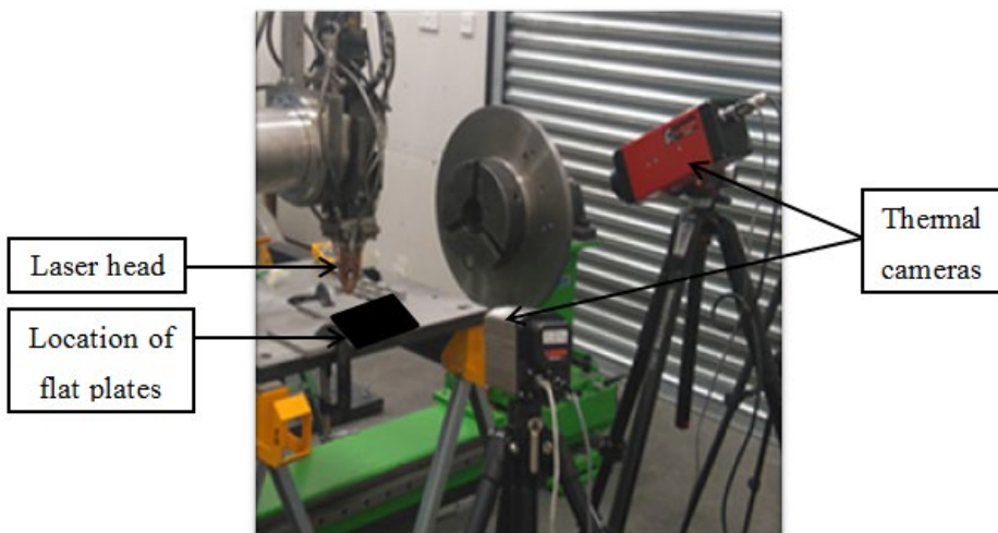
Land thermal cameras used to record the temperatures during the development of the LMD overlay process parameters on flat plates
